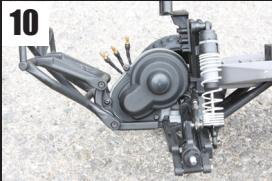
10 Install the gear cover and secure it with the 2 screws.
