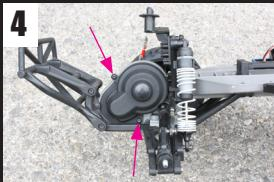
4 Remove the 2 screws holding the gear cover and remove the gear cover.
