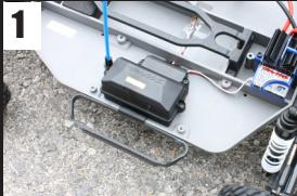
1 Remove the 4 screws holding the receiver box covers and remove the covers.
