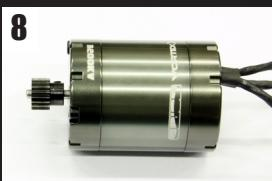
8 Install the pinion gear on the motor, leave a 1.5-2mm space between the motor and the pinion.
