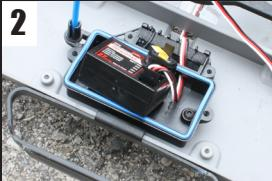
2 Detach the receiver from the box, disconnect the ESC servo lead and pull it out from the box.
