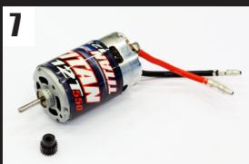
7 Remove the pinion gear from the stock motor.
