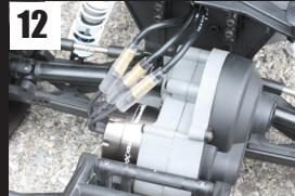
12 Route the wires through the rear shock tower and connect them to the motor following the color codes on the wires.
