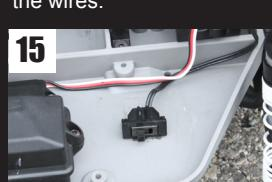
15 Attach the ESC power switch to the chassis using the double-sided tape.
