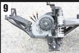
9 Install the motor on the car, adjust the gear mesh and tighten the motor screws.
