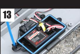
13 Connect the ESC servo lead to the channel 2 of the receiver and attach the receiver to the box.
