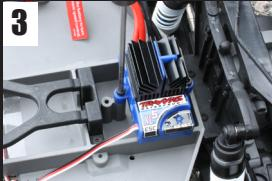
3 Disconnect the motor wires, remove the 2 screws holding the ESC and remove the ESC.
