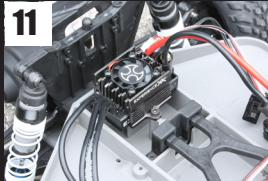
11 Install the ESC and secure it to the chassis using the 2 screws.
