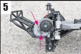
5 Remove the 2 screws holding the motor.
